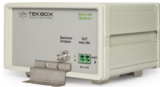
Figure 4: TEKBOX 50 \mu H LISN. Characteristics: DUT max. 16 A, SOURCE max. 250 V, DC/AC Power Supply, frequency range: 9 kHz-100 MHz. Datasheet . This LISN can also be used for testing the DUT used with AC power input and can be used for testing wider range of DUT.
