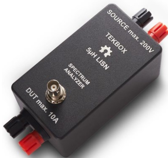
Figure 3: Batronix TEKBOX 5 \mu\text{H} LISN. Characteristics: DUT max. 10 A, SOURCE max. 200 V, DC Power Supply, frequency range: 100 kHz-110 MHz. Datasheet . This 5 \mu\text{H} LISN has very close input impedance curve as the ECSS [1] LISN, so it is sufficient for AcubeSAT project.
